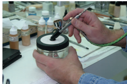
FIGURE 10-27: A CLEANING STATION
